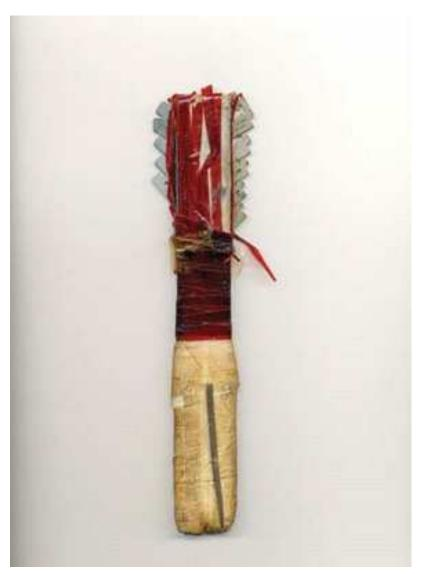
**Materials:** Wood strip; five large razor blades glued into one side; six small razor blades glued into other and wrapped with boxing tape, rubylith and clear tape; handle wrapped with boxing tape.
